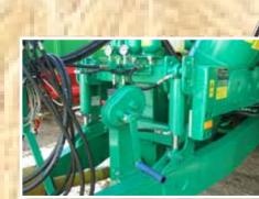
Hydraulic drawbar suspension Extremely robust design improves driving comfort and reduces the impact load on vehicle and driver.
