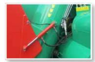
Hydraulic-swivel discharge chute The hydraulic-swivel discharge chute allows precision filling of haulage vehicles.
