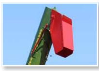
Hydraulic-swivel discharge chute The hydraulic-swivel discharge chute allows precision filling of haulage vehicles. (optional)
