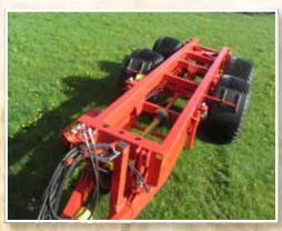
Body-swap running gear The HAWE body-swap system enables you to exploit your high-quality tandem or tridem running gear to the full. Matching grain bodies are available from between 25 to 38 m<sup>3</sup> capacity.
